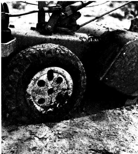
Fig. 1. A small tractor wheel caked with mud and mud that has been thrown on the tractor chassis.
