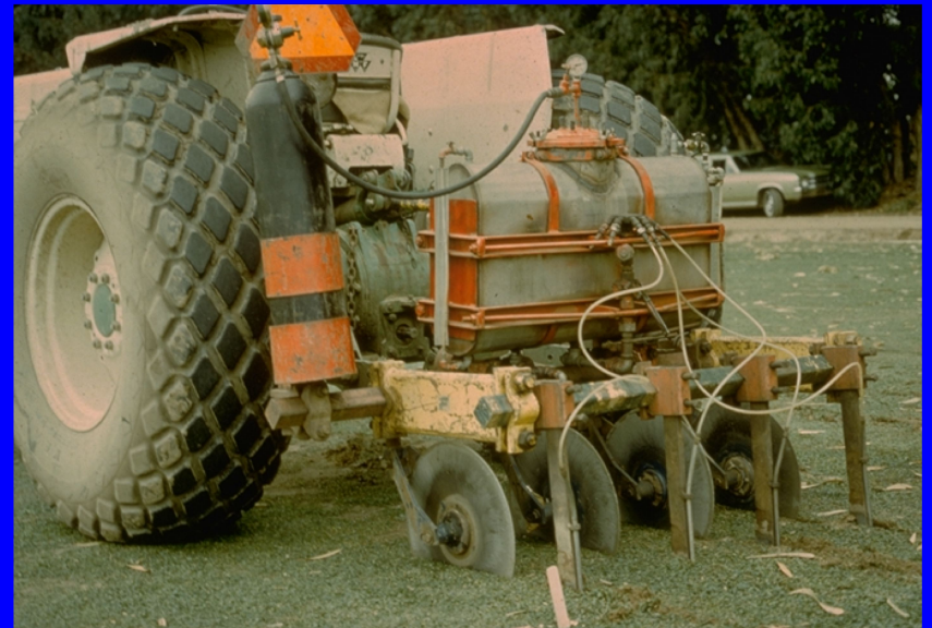
TURF GRASS INJECTION WITH COULTER CUTTERS
